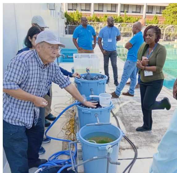
Ecological Purification Systems (EPS), Slow Water Filtration demonstration by Dr. Nobutada Nakamoto
